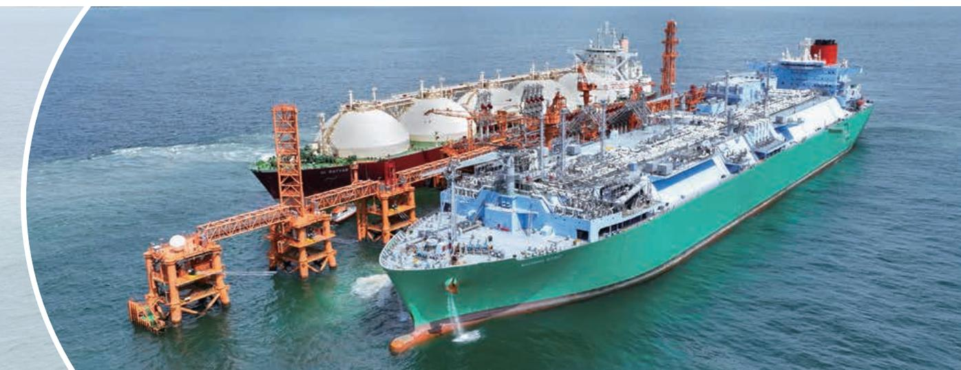
An LNG shipment (left) arrives at Hong Kong's first offshore LNG terminal, and is loaded onto the floating storage and regasification unit vessel (right), the Bauhinia Spirit, for regasification.
