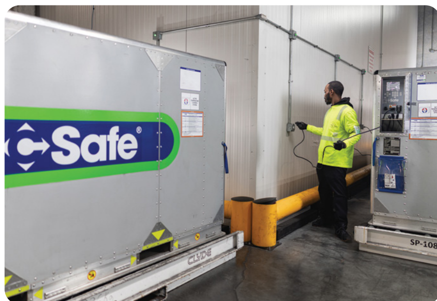
Chicago ORD building 838 A handler plugging in a self-temperature contained active container for temperature sensitive cargo.
